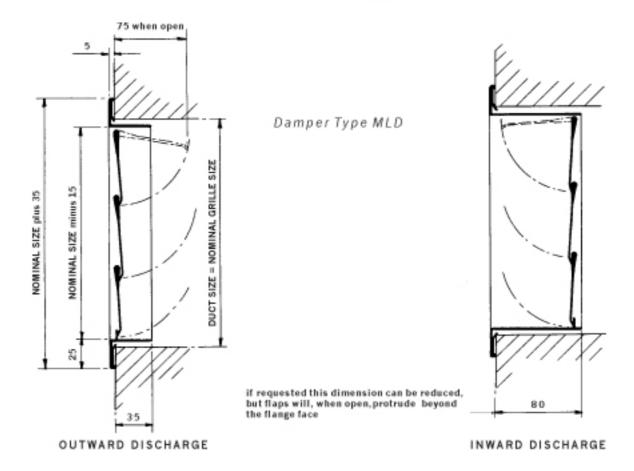
TYPE MLD plastic faced Multi-Leaf pressure relief damper consists of a single set of horizontal light gauge plastic flaps mounted on stainless steel axles pivoting about their top edge which swing open under slight air pressure, the amount of opening being dependent upon the quantity of air being discharged in relation to the size of the damper.
